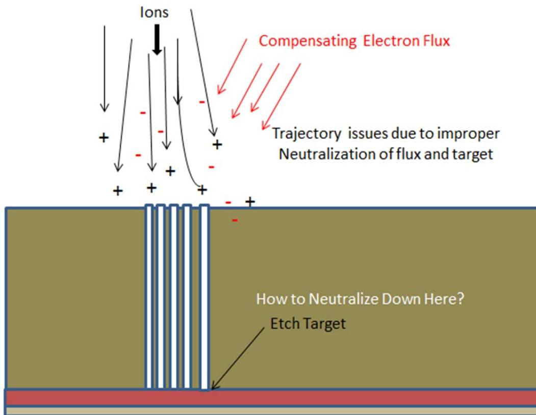
Figure 1. High aspect ratio etching with traditional charged particle technology.
