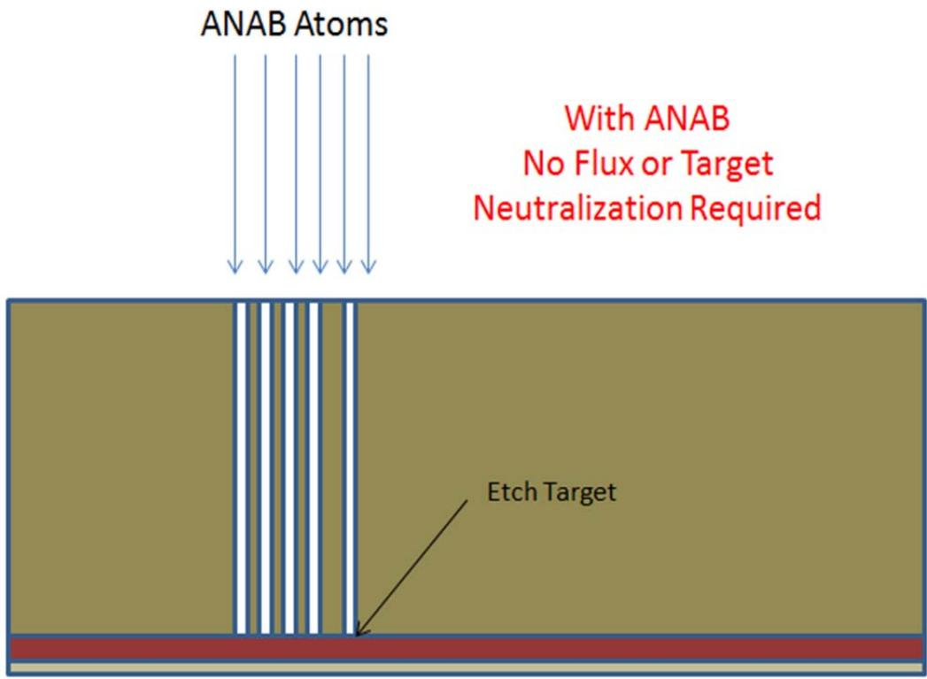
Figure 2. High aspect ratio etching with Accelerated Neutral Atom Beam technology
