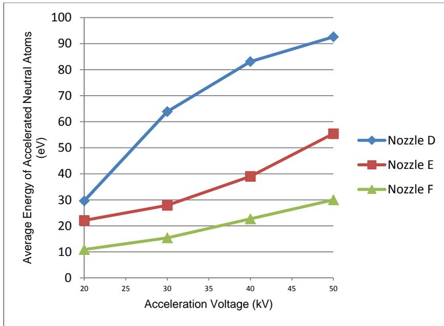
Figure 4. ANAB energy vs. acceleration voltage
