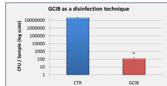
Graph 1. Study 3 validation results from an outside vendor show a 5 log reduction in bacterial CFU/sample by GCIB treatment as compared to controls (\* p<0.0001).
