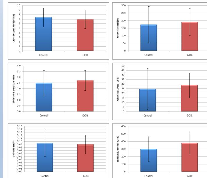
No significant differences are found between fresh-frozen control goat flexor tendons to GCIB processed tendons in any of the mechanical testing properties. Cross section area, p=0.56; Ultimate load, p=0.64; Ultimate elongation, p=0.52; Ultimate stress, p=0.53; Ultimate strain, p=0.75; Tangent modulus, p=0.16.
