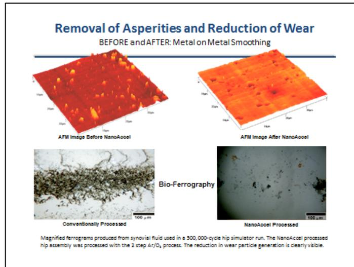
Fig. 3 – Removal of asperities and reduction in wear particles
