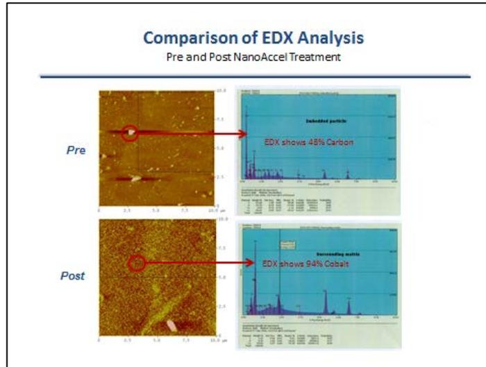
Fig. 4 – Carbon debris pre and Post NanoAccel treatment
